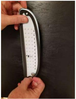
Install lens. You may find it easier to place the screws thru the lens and stack the LED board on top, using the screws to hold the lens and LED board in alignment.
