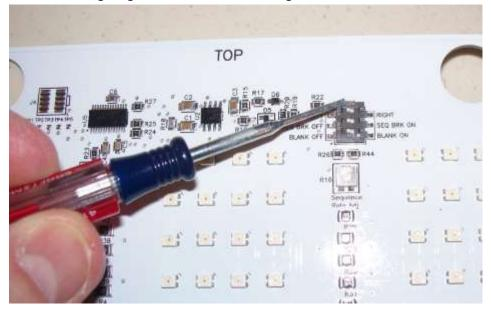
Turn on the turn signal and adjust the sweep rate on each board by turning the potentiometers R16. Adjust R16 Counter clockwise (CCW) for slower, clockwise (CW) for faster.
