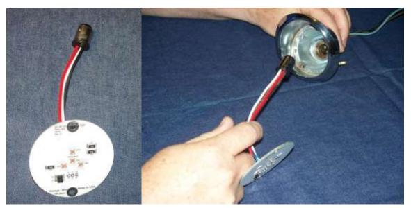
Push in with a flat blade screwdriver and turn clockwise.
