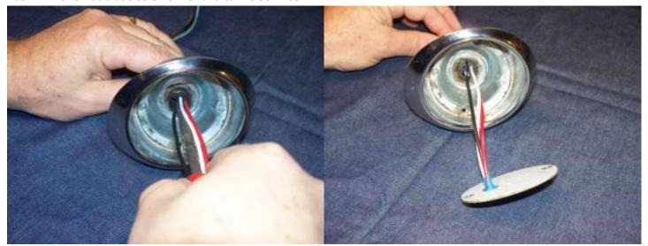
With the wires in the housing, twist them into a small loop and push into the housing.
