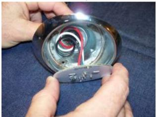
With the wires twisted, push the board to the bottom of the housing. Make sure that you do not pinch any of the wires under the board.
