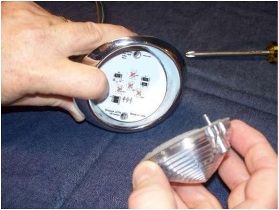
Tighten the lens screws.
