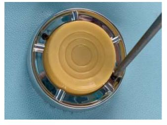
Remove the screw the single screw that hold the reflector to the roof. Keep this screw you will need it later.
