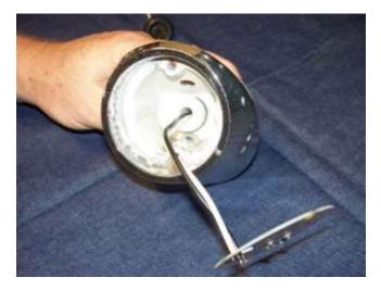
Install the gasket and lens. I have found it easier to assemble the lens, gasket board and screw as one assembly.
