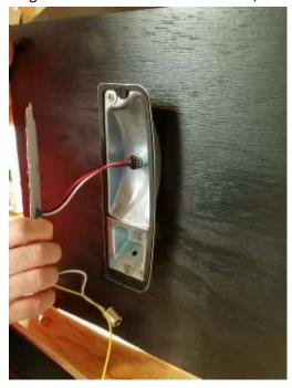
Plug 1156 cable to brake socket. Black and White wires.
