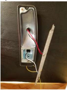
If you have the amber turn option, then you will need to drill a small hole in the light housing for the yellow wire. Make sure you add a gromet to keep the wire from chafing. The yellow wire will need to be connected to the turn signal circuit. Preferably to the front turn signal because it is separate from the rear brake circuit. No need for an extra ground wire. As long as there the brake and reverse cables are connected, there is a connection to ground.
