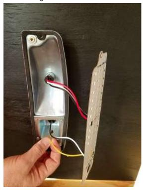
You may find it easier to use the lens screws to hold the LED board in alignment.
