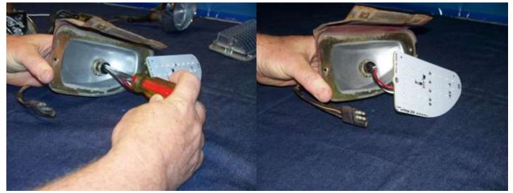
Install the gasket and lens. I have found it easier to assemble the lens, gasket board and screw as one assembly. The screws are a tight fit to the circuit board and can be drive thru with a screwdriver. Make sure that you do not pinch any of the wires under the board.
