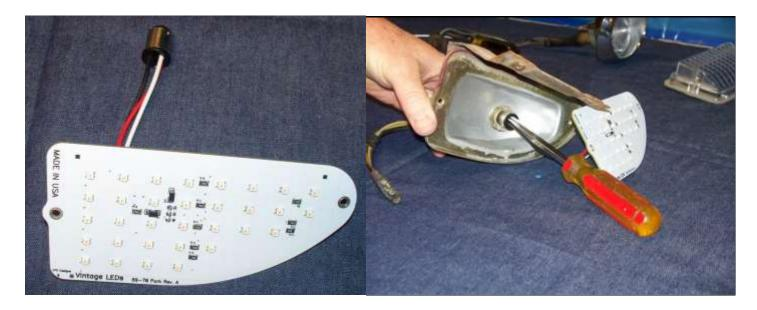
Push in with a flat blade screwdriver and turn clockwise.
