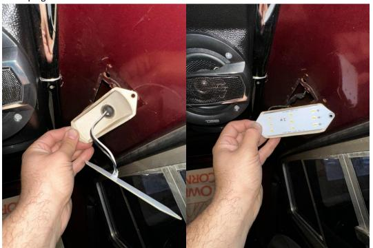
Place lens over LED board. Insert screws to align Lens to LED board and light assembly.
