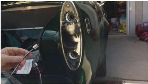
There as slot in the back of each plug for a flat head screw driver. Align the locking pins and rotate clockwise.
