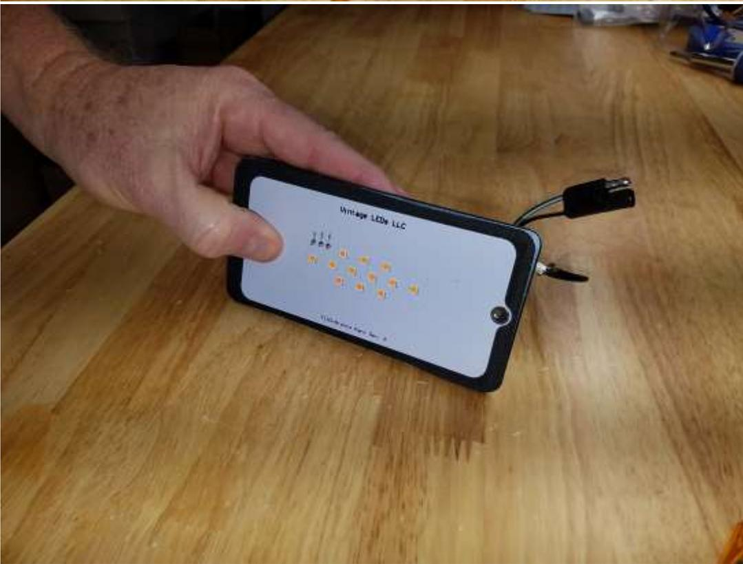
You may find it easier to use the lens screws to hold the LED board in alignment.
