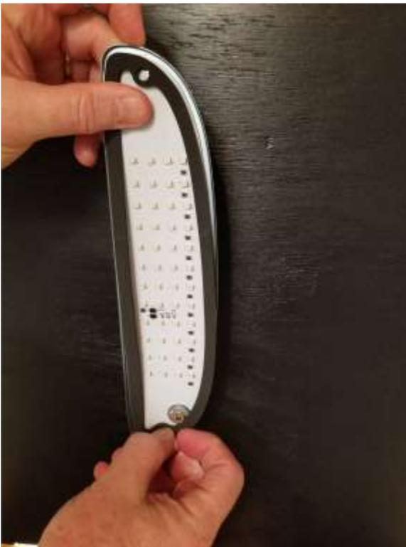
Install lens. You may find it easier to place the screws thru the lens and stack the LED board on top, using the screws to hold the lens and LED board in alignment.
