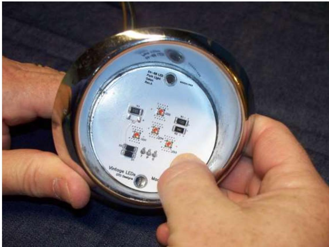
Install the gasket and lens. I have found it easier to assemble the lens, gasket and screw as one assembly. For extra insurance against leaks, you can add a gasket below and above the LED board
