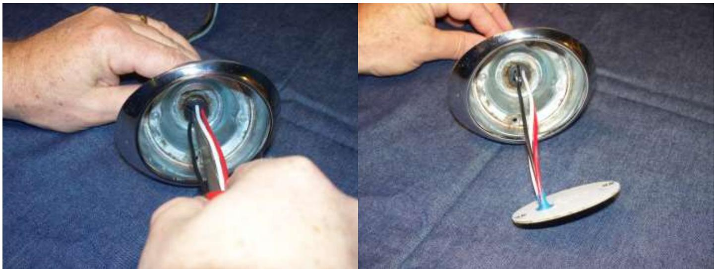
With the wires in the housing, twist them into a small loop and push into the housing.
