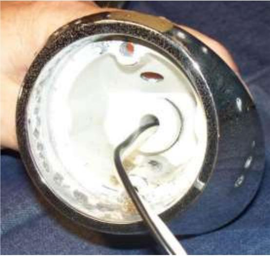
Pull the two wires thru the hole. Add a grommet to seal the hole.
