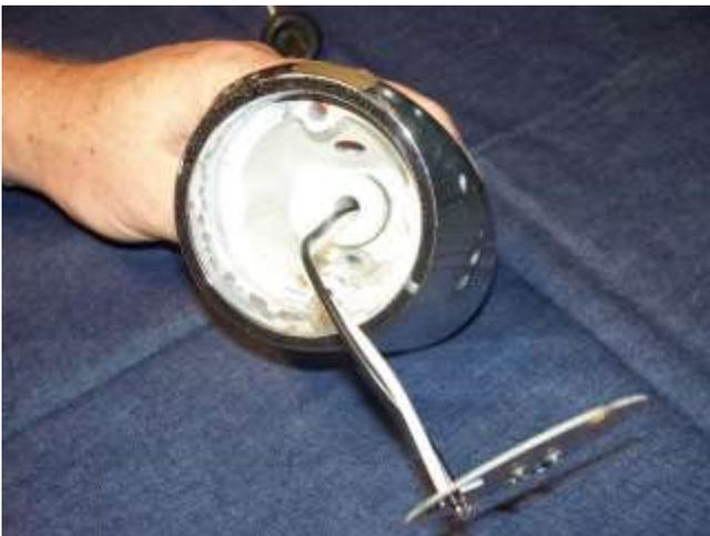
Install the gasket and lens. I have found it easier to assemble the lens, gasket board and screw as one assembly.
