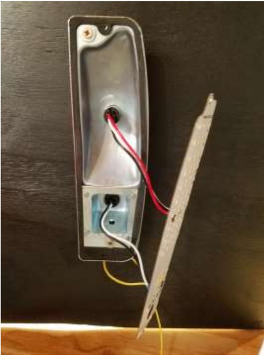
If you have the amber turn option, then you will need to drill a small hole in the light housing for the yellow wire. Make sure you add a grommet to keep the wire from chafing. The yellow wire will need to be connected to the turn signal circuit. Preferably to the front turn signal because it is separate from the rear brake circuit. No need for an extra ground wire. As long as there the brake and reverse cables are connected, there is a connection to ground.
