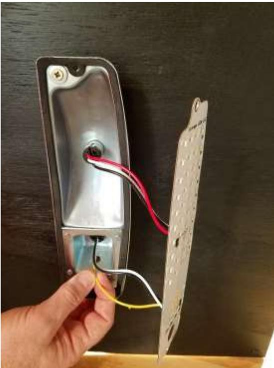
You may find it easier to use the lens screws to hold the LED board in alignment.
