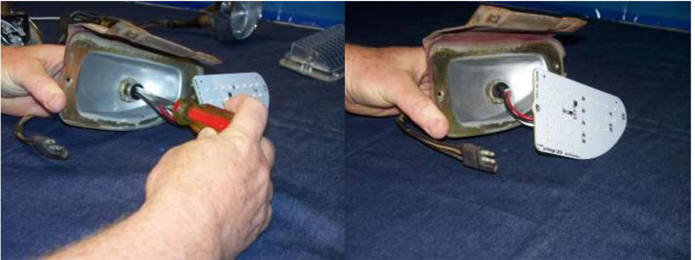
Install the gasket and lens. I have found it easier to assemble the lens, gasket board and screw as one assembly. The screws are a tight fit to the circuit board and can be drive thru with a screwdriver. Make sure that you do not pinch any of the wires under the board.
