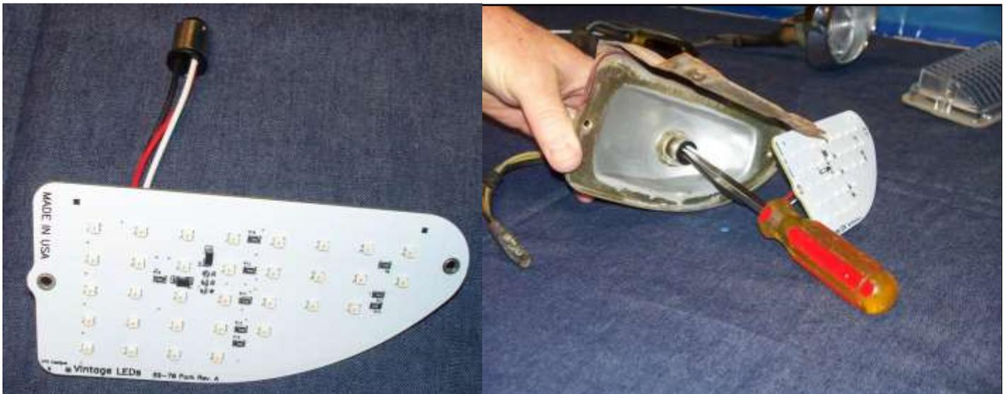
Push in with a flat blade screwdriver and turn clockwise.
