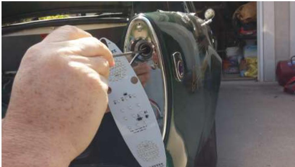
Same procedure for the 1157 socket, note that the 1157 socket has offset locking pins.
