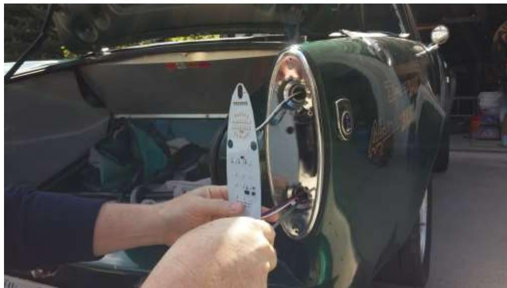
Curl up the excess wire and push it in to the bulb sockets. The LED board need to sit flush against the light housing.
