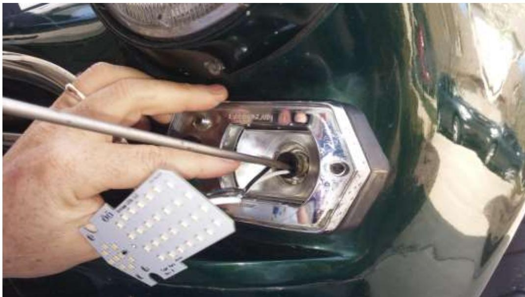
Press the board against the light housing. There are alignment slots above the white LEDs. The turn LEDS should fit inside the cavity where the bulb was.
