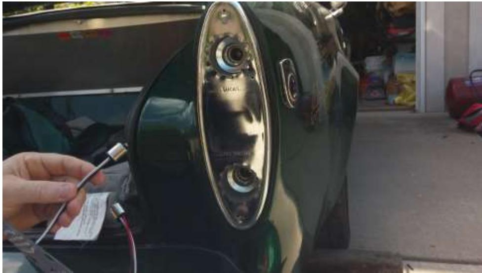
There is a slot in the back of each plug for a flat head screw driver. Align the locking pins and rotate clockwise.
